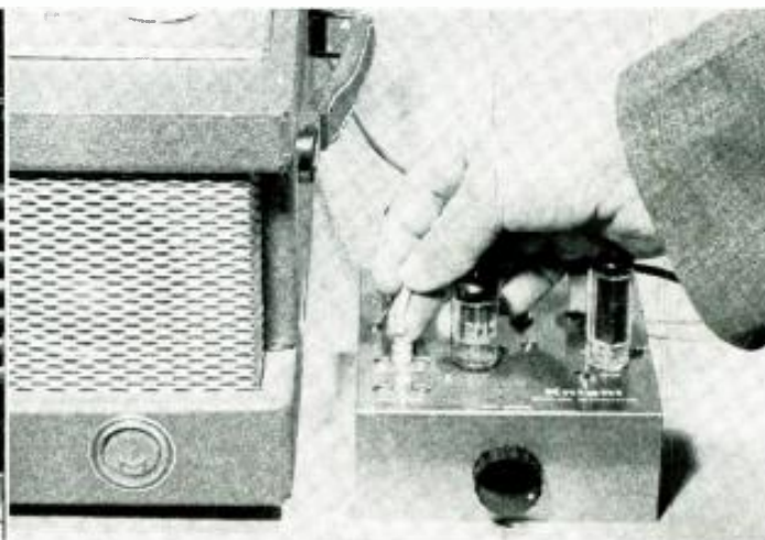
The second channel from a recorder with stereo playback may be plugged into the unit for broadcast to a nearby radio.
