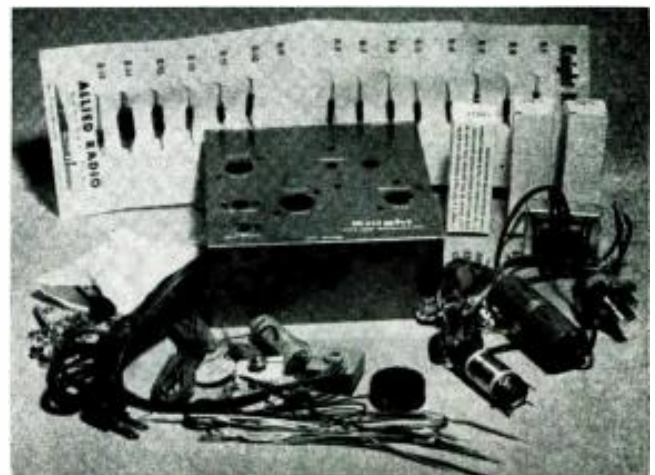
The Allied Radio Wireless Broadcaster Kit as it comes from the package. The resistors are all marked and arranged on a card.
